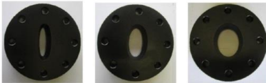
Figure 2. Different geometries for the upper die with a major axis of 64mm and a minor axis of 16mm, 32mm et 48mm respectively.
