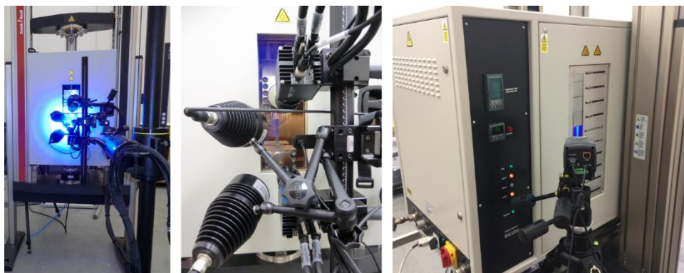
Figure 1. The experimental set-up including DIC and infrared camera.
