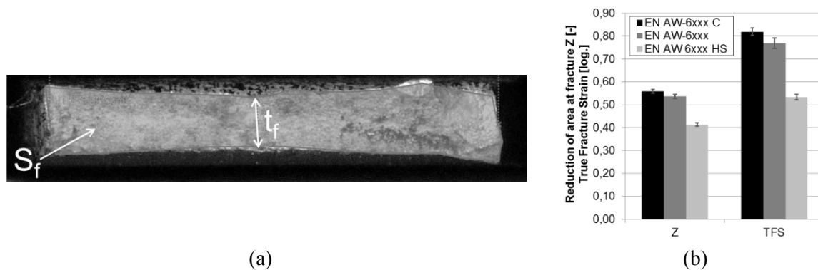
Figure 3. (a) Fracture surface measurement (b) Results gained by fracture surface measurement
