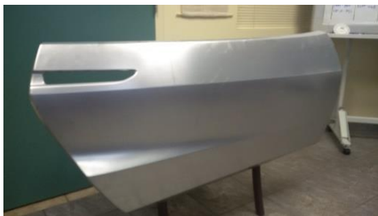
Figure 18. Door outer, A6022-T4, t1.2mm.
