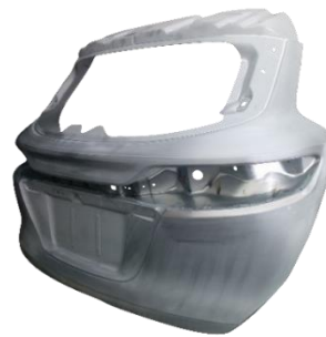
Figure 16. Liftgate, CR4, t0.6mm..
