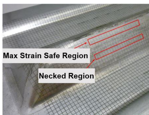
Figure 21. Necked and maximum safe strain regions of the DP600 EHDF specimen [6].
