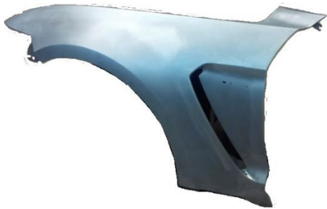
Figure 15. Fender, A6022-T4, t1.0mm.
