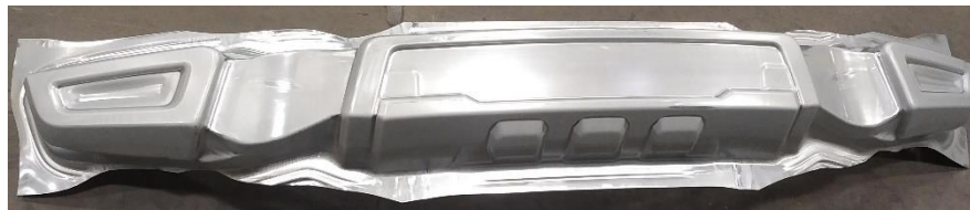
Figure 17. Front bumper, EDDQ, t1.86mm.
