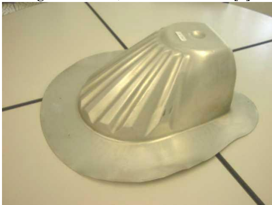
Figure 13. Reflector, A1080-0, t1.2mm[5].
