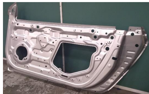
Figure 19. Door inner, A6022-T4, t1.2mm.
