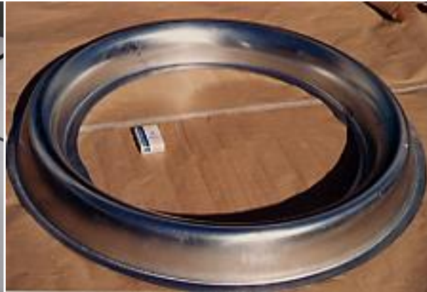
Figure 12. Jet engine lip skin, A2219-0, t1.6mm[5].
