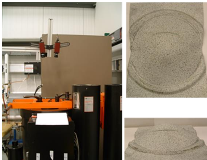
Figure 3. Experimental setup for determination of FLC_0 using DIC showing samples exhibiting necking and fracture.
