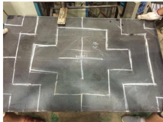
Figure 14. Heating lines of sail plate
