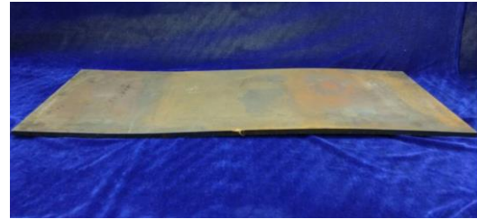
Figure 16. Forming test for S curved plate.
