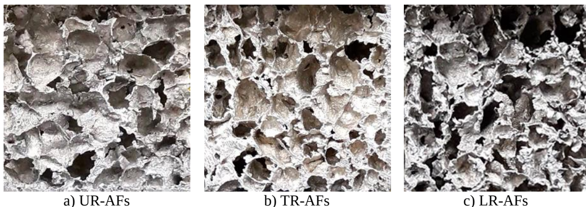
Figure 2. The macrostructure morphology of the investigated composite foams
