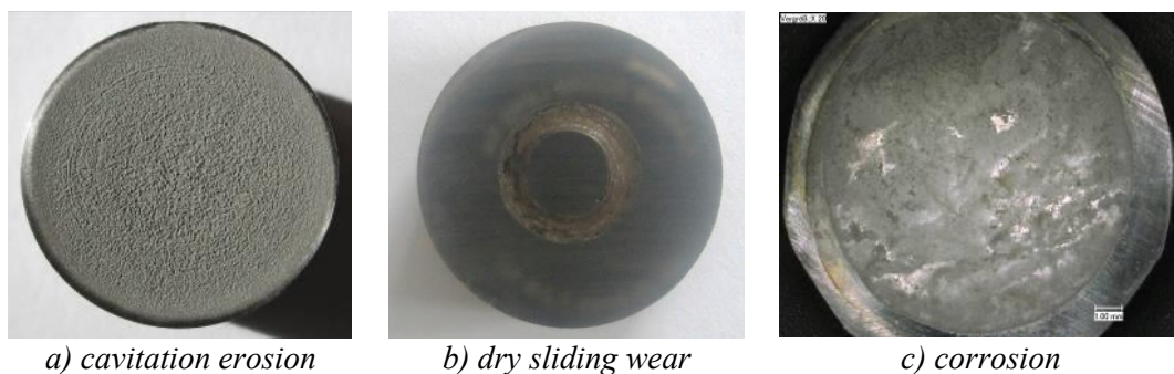
Figure 7. Images of wear and corrosion of the sample surfaces after the tests.
