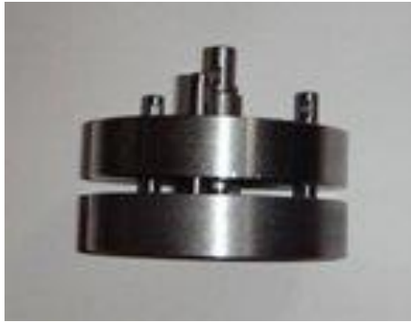
Figure 1. Specialised device for bearing balls compression test
