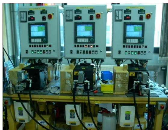
Figure 3. Fatigue testing machine for bearing balls
