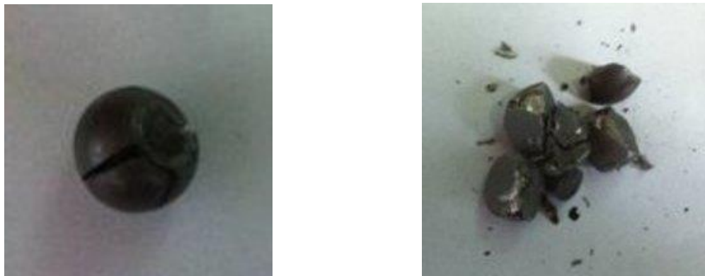
Figure 5. Ball tested at compression
