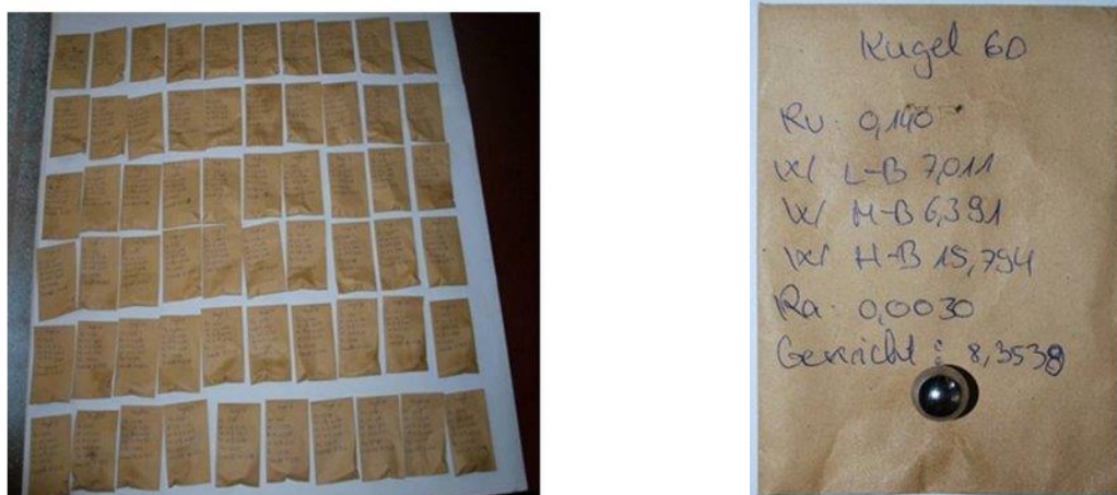
Figure 7. Bearing balls D_w = 12,7 mm after n = 200 \cdot 10^6 rotations
