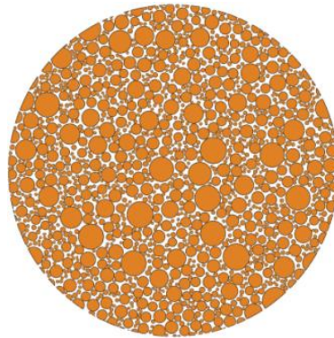
Figure 2. A 2D cylindrical model for simulating indirect tensile fatigue test
