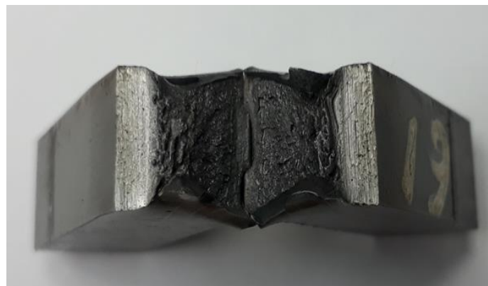
Figure 9. Halves of broken Charpy V-Notch Impact specimen.
