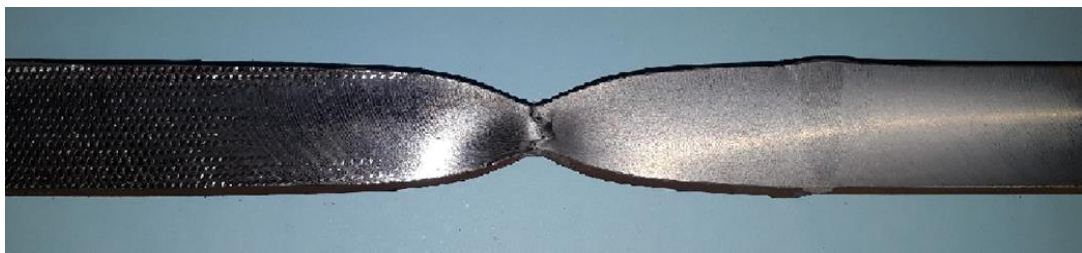
Figure 5. Fracture location of the tensile strength test specimen.
