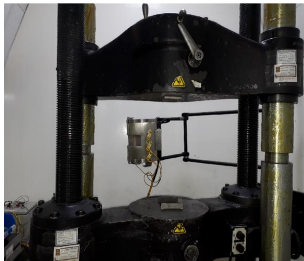
Figure 4. Universal machine type Satec 5500R 200BTE.
