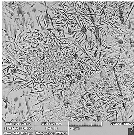
a) Martensite structure of the alloy
