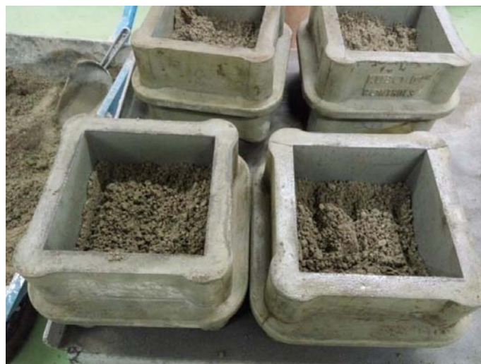
Figure 1. Preparing cubic samples
