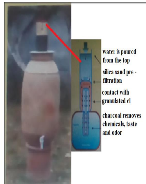
Figure 4. Schematic diagram of three stage portable water filter.
