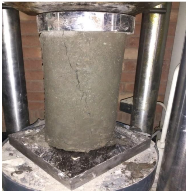
Figure 3. Compression test of concrete cylinder under observation
