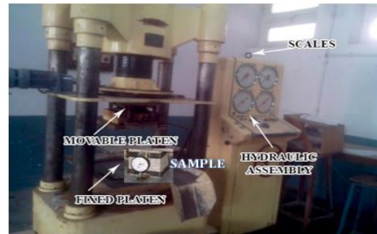
Figure 1: Test setup and test sample
