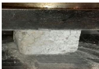
Figure 5. Bulging during Compression Test
