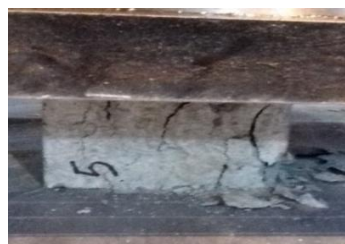
Figure 6. Spalling compression test
