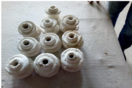
(a) Casted specimen; unfired, unglazed and unfelted.
