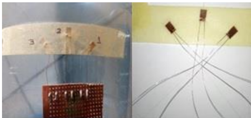
Figure 1: A set of strain gage sensors assembled at an angle of 45 degrees apart (LHS) and glued to the plastic digester (RHS)
