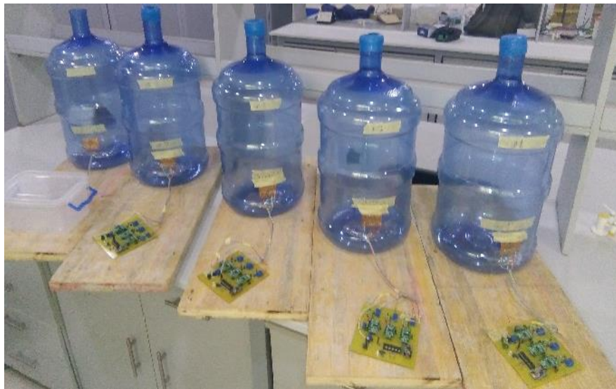
Figure 3: Digester plastic before loading it with feedstocks. Attached to the lower side of the plastics are the strain gages which are connected to the data acquisition board placed in front of the digester
