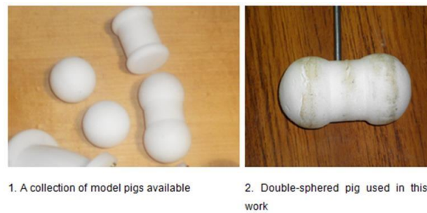
Fig. 4 Model pigs used for the pigging study
