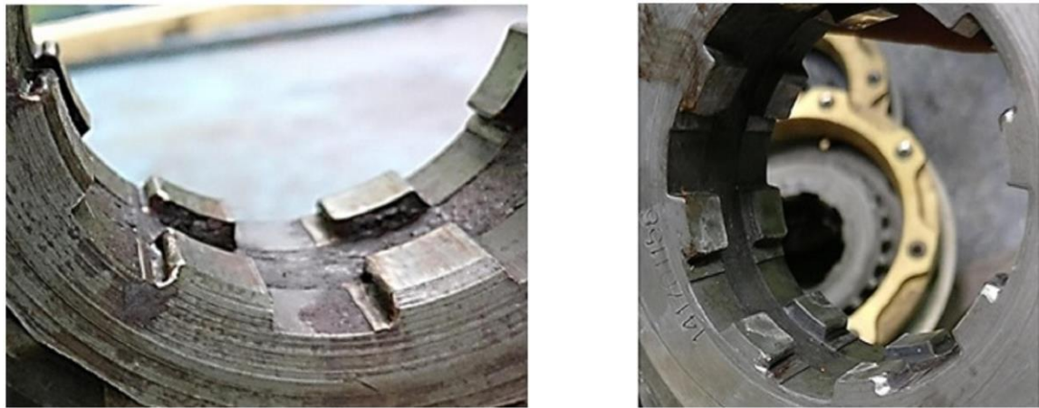
Fig. 1. Wear of internal splines of the synchronizer carriage of IV-V transmissions of KAMAZ gear change box
