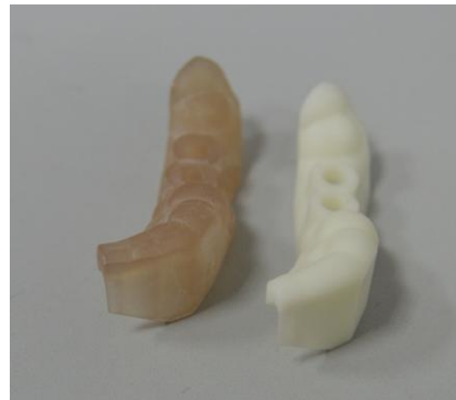
Figure 3 - The finished guide is made of plastic on the CNC mill (left). On the right - a guide, made with RSPro 600 of a photopolymer.
