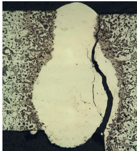
Figure 1. General view of the CGI plates weld 30 (left) and CGI 35, magnification x 50, (grinding is etched)
