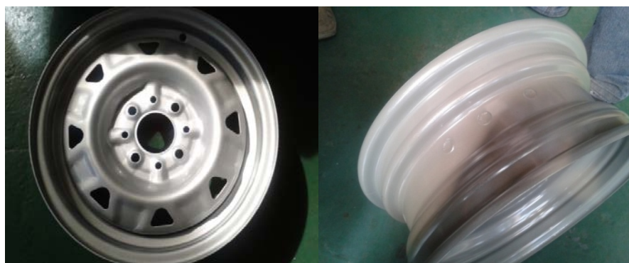
Figure 5. Stamped wheel from pilot run of pickled temper-rolled strip of 07GBYu steel for the LADA automobile of JSC Avtovaz.
