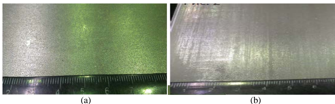
Figure 4. Tempered strip surface of pilot run (a) and non-tempered strip surface of batch (b).
