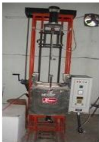
Fig.1: Bottom Pouring Furnace
