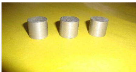
Fig.6 Specimen before compressive test
