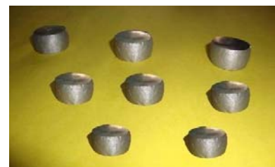
Fig.7 Specimen after compressive test
