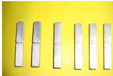
Fig.3 Specimen before impact test
