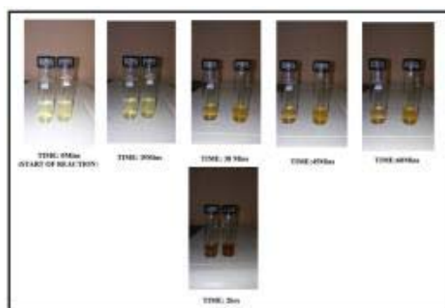
FIGURE 1a : Color change during production of Silver Nanoparticle with time.
