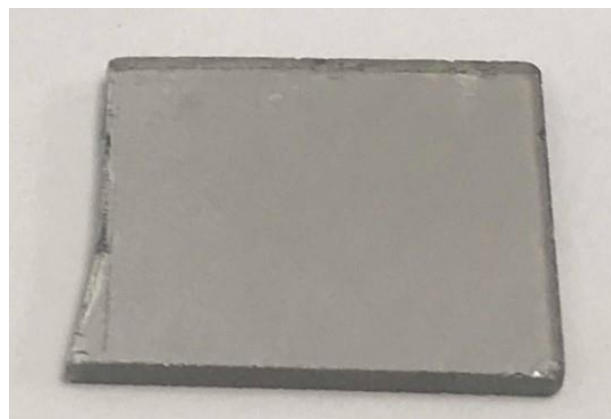
Figure 2. The GO thin film on glass substrate prepared by SPT
