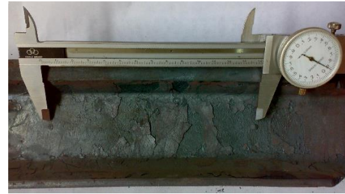
Figure 9. Figure 10. Measurement of hump marks on the web of rail
