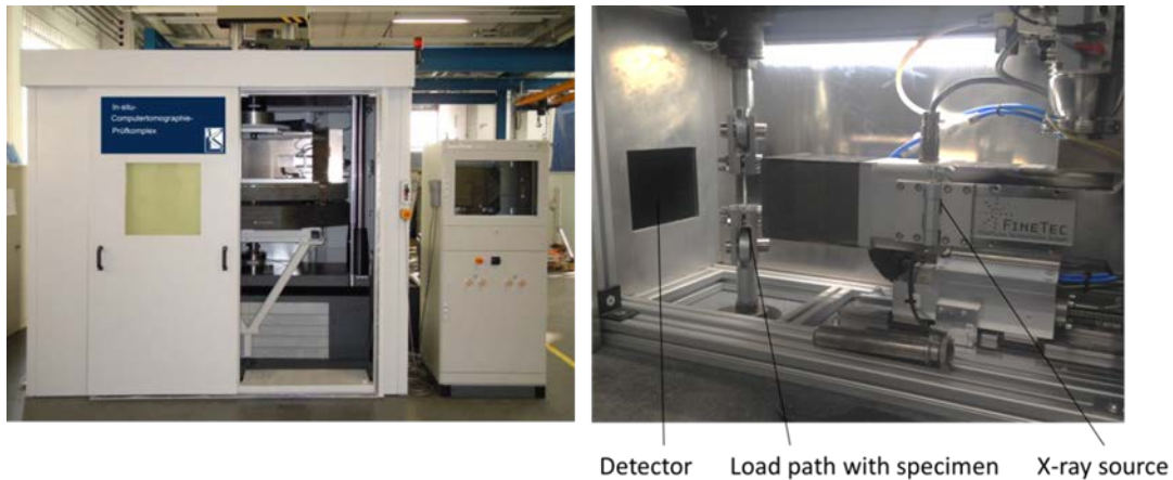
Figure 2. In-situ CT test rig (left) and test unit (right)
