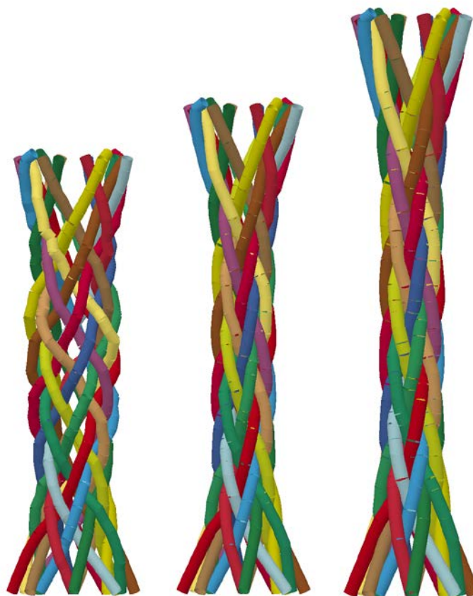
Figure 6. Stages of the simulation of tensile test of the tubular braid
