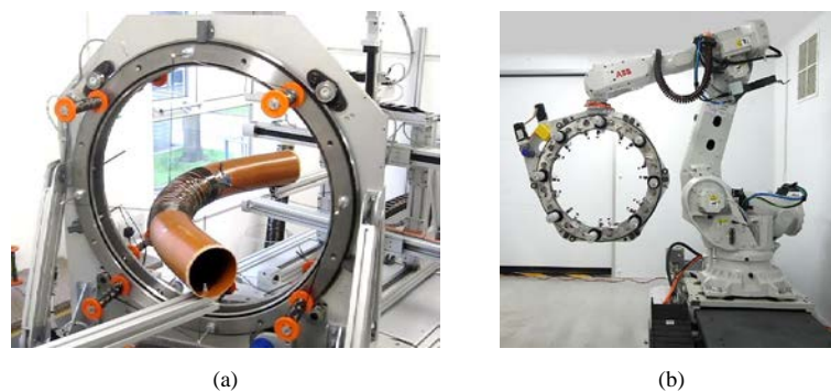
Figure 11. (a) Prototype multiaxis winding developed at the University of Manchester (b) The multi-axis winding concept used in commercial equipment developed by Cygnet Texkimp UK Limited
