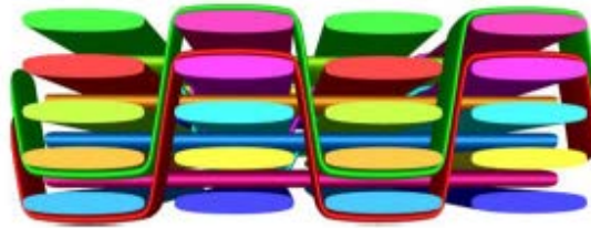
Figure 4. Reinforcement with the binder path optimised to achieve maximum buckling coefficient
