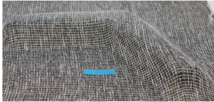
Figure 9. Formed sample with the L-Profile forming device for the biaxial reinforced weft-knitted fabric
