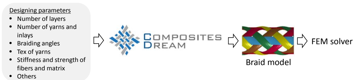
Figure 10. Analysis procedures for braided composites tubes using Composites Dream
