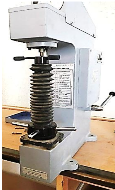
Figure 5. The Brinell hardness test
