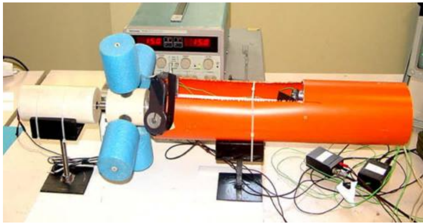
Figure 5. Chiral rotor prototype with 4 smooth surface rotating cylinder blades [25]
