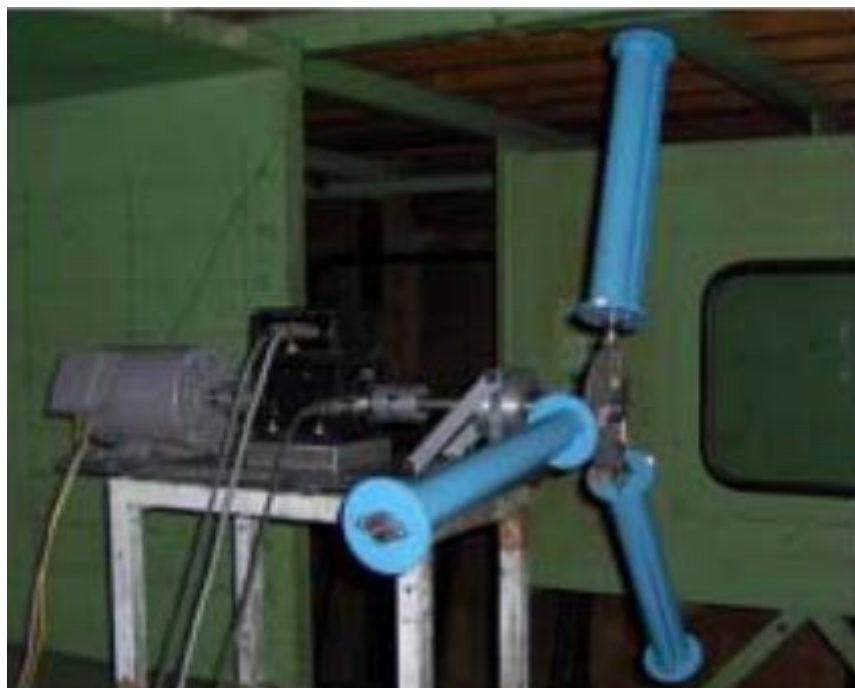
Figure 6. MWT with Savonius shaped as cylinder blades [27]
