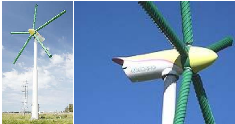
Figure 1. Magnus wind turbine with fin-like on rotating cylinder blades [13]
