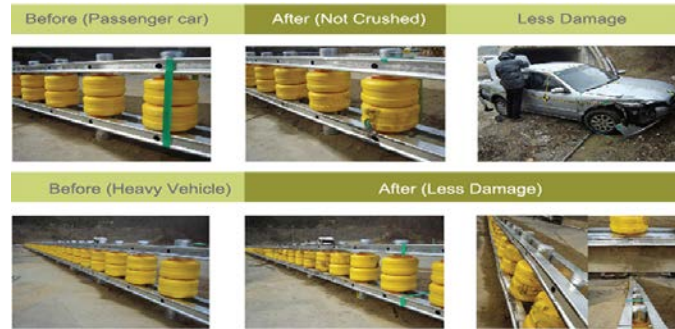
Figure 6. Crash test for car and truck collision at RB (KSI Korea).[8]
