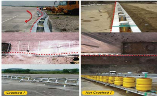
Figure 5. Crash test comparison between conventional barriers and RB (KSI Korea).[8]
