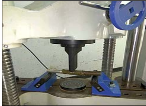
Fig 5: Specimen under three-point bending
