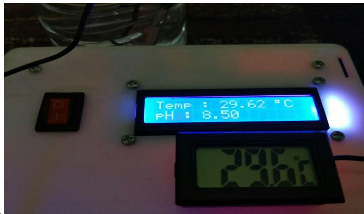
Figure 4. Testing temperature sensor DS18B20 waterproof.
