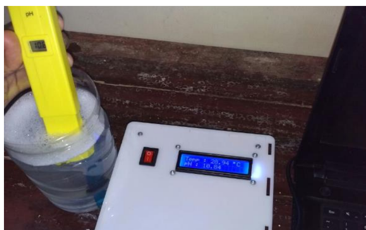
Figure 5. Testing pH meter analog kit sensor.
