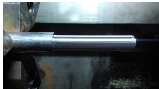
Figure 4. Shows smooth finish at higher cutting speeds
