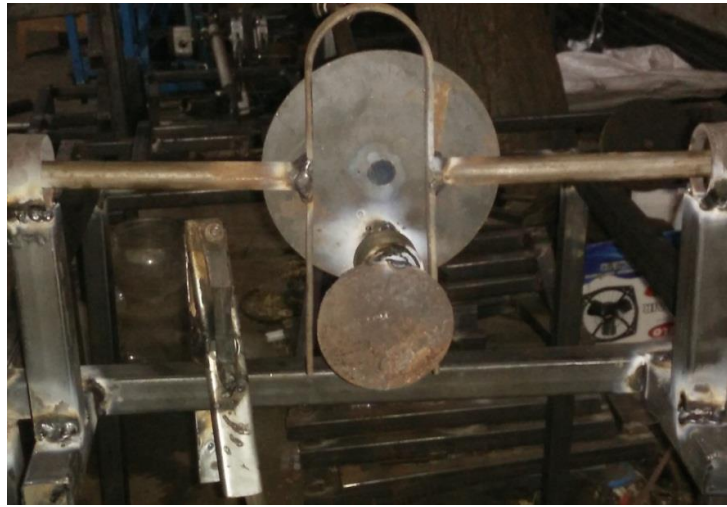
Figure 12. Scotch Yoke Mechanism used
