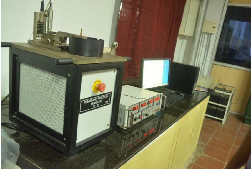
Figure 1. Wear and Friction test experimental set up with specimen
