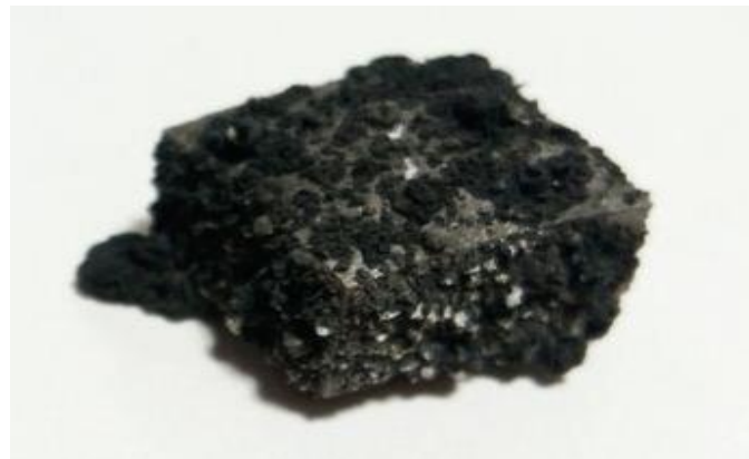
Figure 4. Sample with burnt magnesium after foaming is done.
