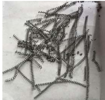
Figure 6. Long continuous chips.
