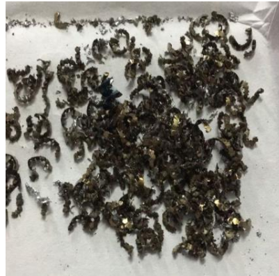
Figure 8. cubic boron nitride discontinuous chip
