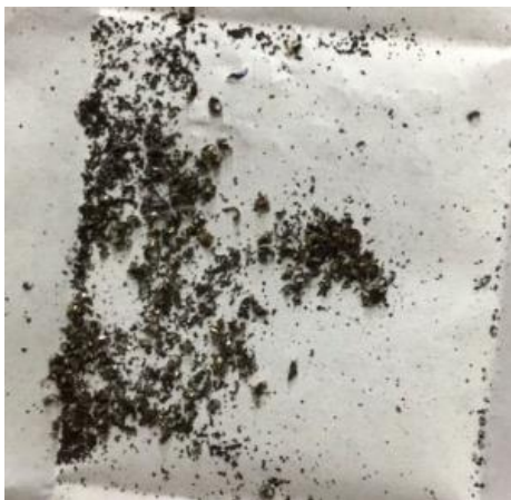
Figure 3. Fine discontinuous chips.
