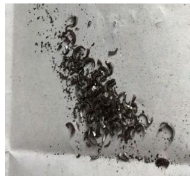
Figure 2. Small discontinuous chips.
