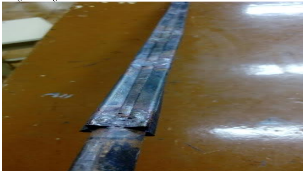
Figure 5. Design of finned tube
