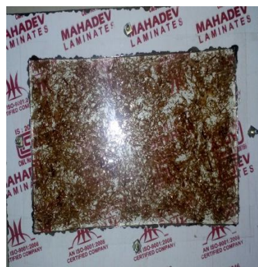
Figure 5. Hand lay-up method
