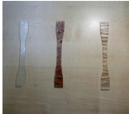
Figure 7. Specimens of dog bone shape for tensile test
