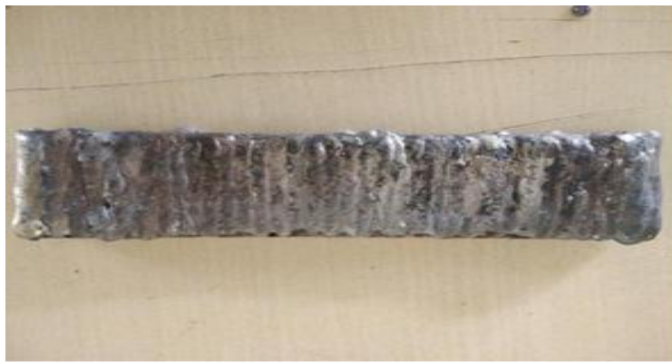
Figure 2. First layer of cladding on base metal
