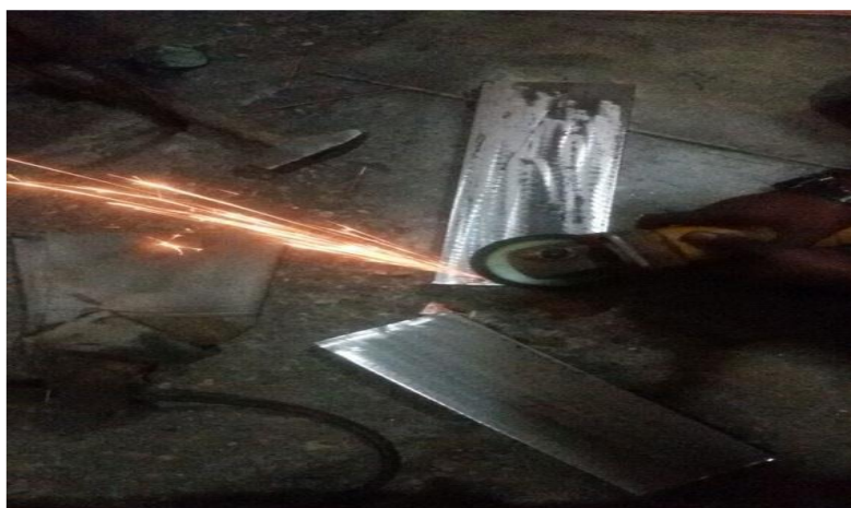
Figure 1. Grinding of base metal to remove impurities
