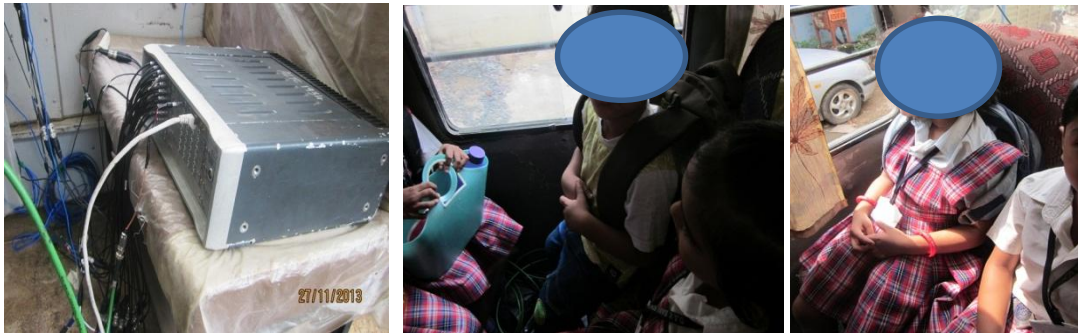
Figure 3. LMS Scadas vibration analyser, Children on the seat pad accelerometer.
