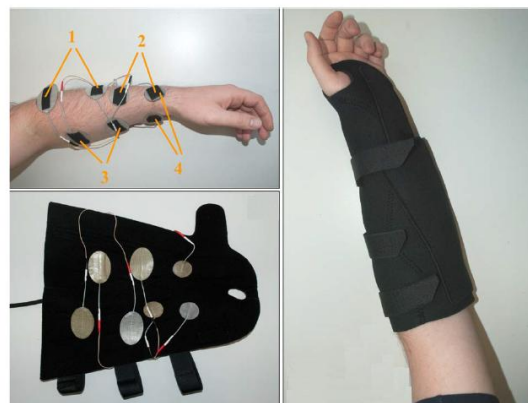
Figure 8. Electrode positions with the assigned channel numbers of the stimulator (Top Left); Electrodes fixed with a velcro strap for easy and quick electrode mounting (Bottom Left); Mounted forearm sleeve (Right).
