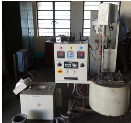
Figure 1. Stir casting set up
