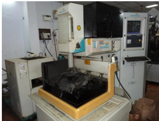
Figure 2. WEDM experimental set up (Electronica Sprint cut)
