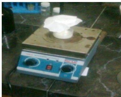
Figure 1. Magnetic Stirrer
