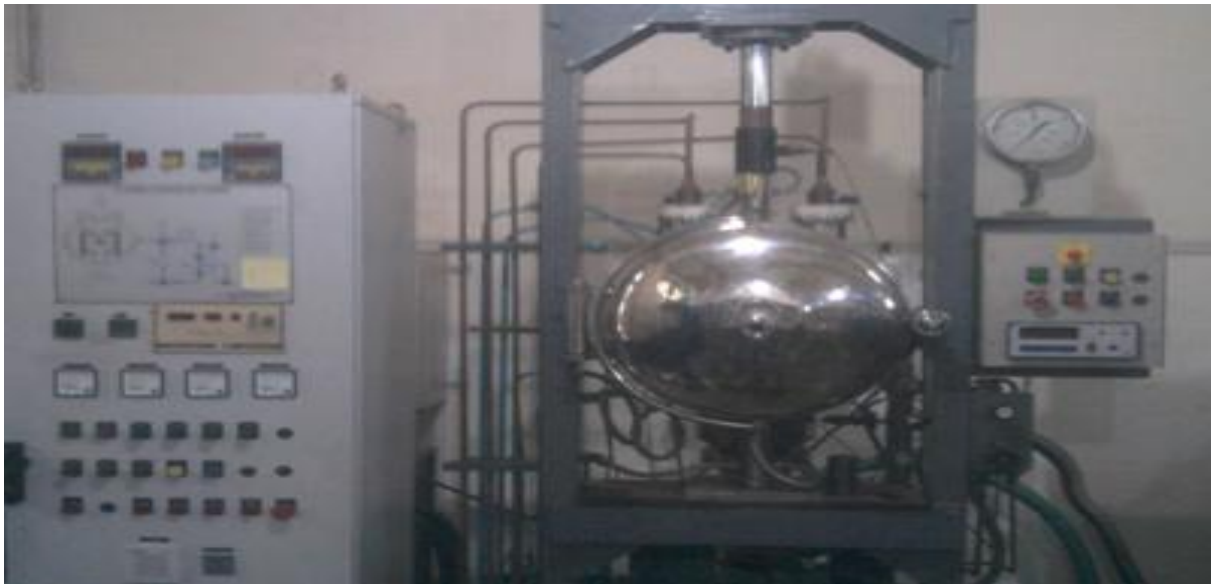
Figure 2. Vacuum hot press diffusion bonding equipment.
